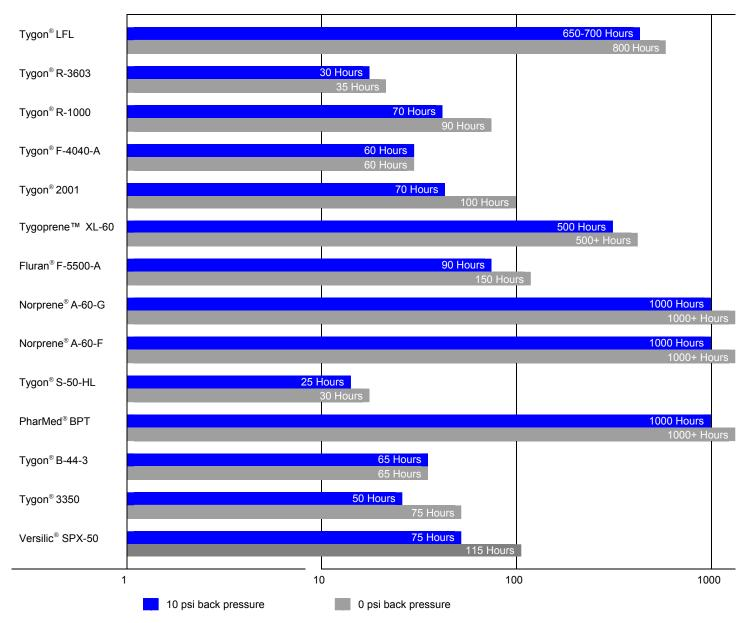
The performance of tubing in peristaltic pumping applications is affected by the conditions of use and equipment utilized, along with size and wall thickness of the tubing tested. The data above is presented for information only and should not be utilized for specification purposes.
