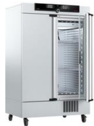
Concrete testing in a climate chamber with CO 2 control
